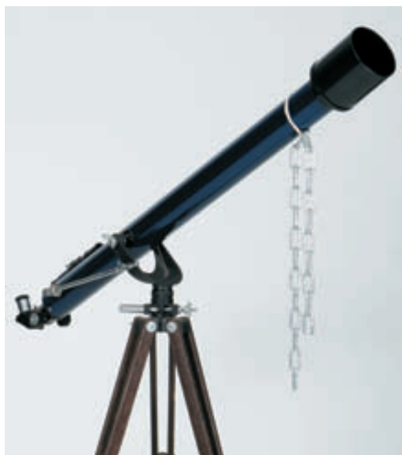
Left: An easy way to improve a tripod's stability is to suspend a weight between its legs. Right: A free-hanging chain is surprisingly good at absorbing vibrations.
