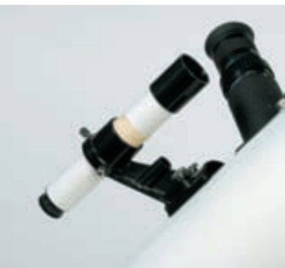
A loose finderscope can often be fixed with a few wraps of tape between the tube and the front end of the holder.
