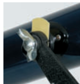
Top: This slow-motion cable is thick and solid. If yours is thin and springy, a radio knob might work better. Bottom: A plastic bread-bag clip makes a handy washer.
