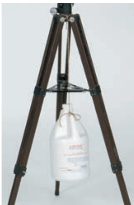
Left: An easy way to improve a tripod's stability is to suspend a weight between its legs. Right: A free-hanging chain is surprisingly good at absorbing vibrations.
